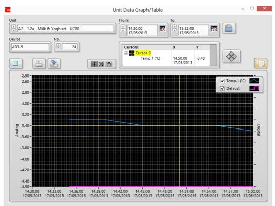
First of all it's necessary to choose the plant unit of which you'd like to retrieve data and set the start and end date and time of the time frame you are interested in. Then press button "Load" at the side of the period end box to load data. To set date and time, press the right hand button in the relative boxes: a window will pop up where it will be easy to choose day, month, year and time.
